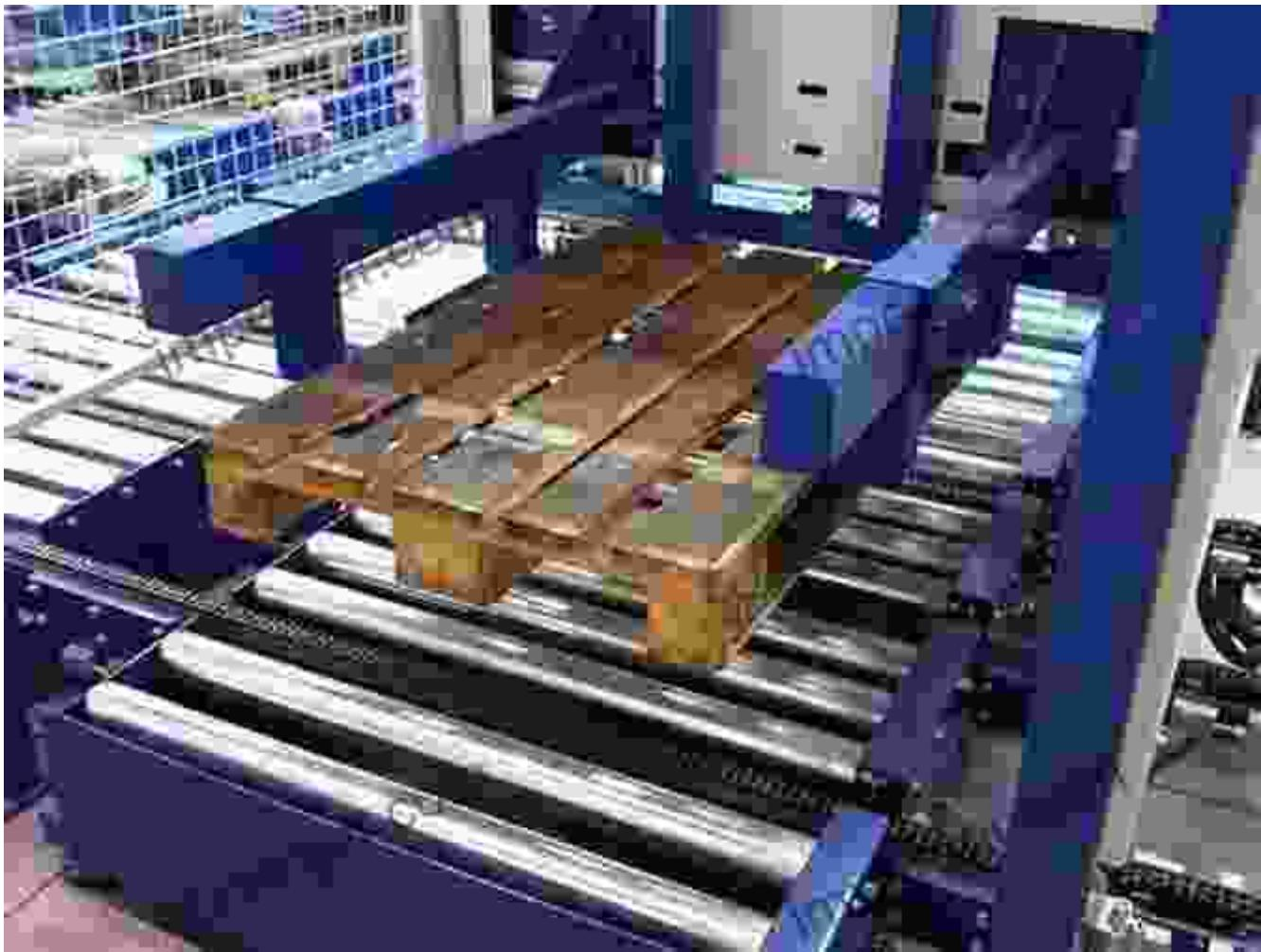
Chain conveyors use a chain with attached flights to move units. They are ideal for applications requiring precise positioning and accumulation.
