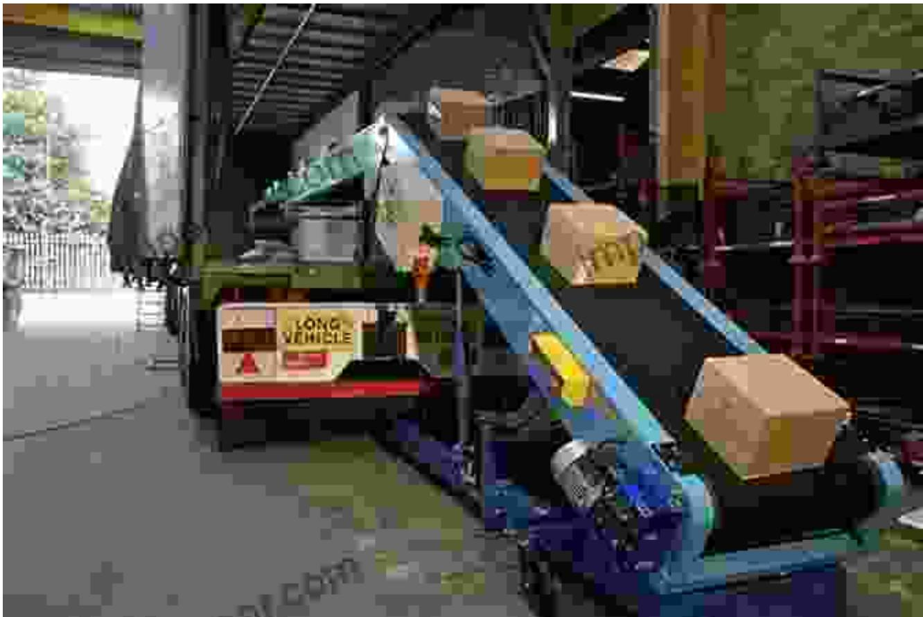
Belt conveyors feature a continuous loop of belt that moves units along a fixed path. They are suitable for a variety of applications, including conveying goods over inclines or declines.
