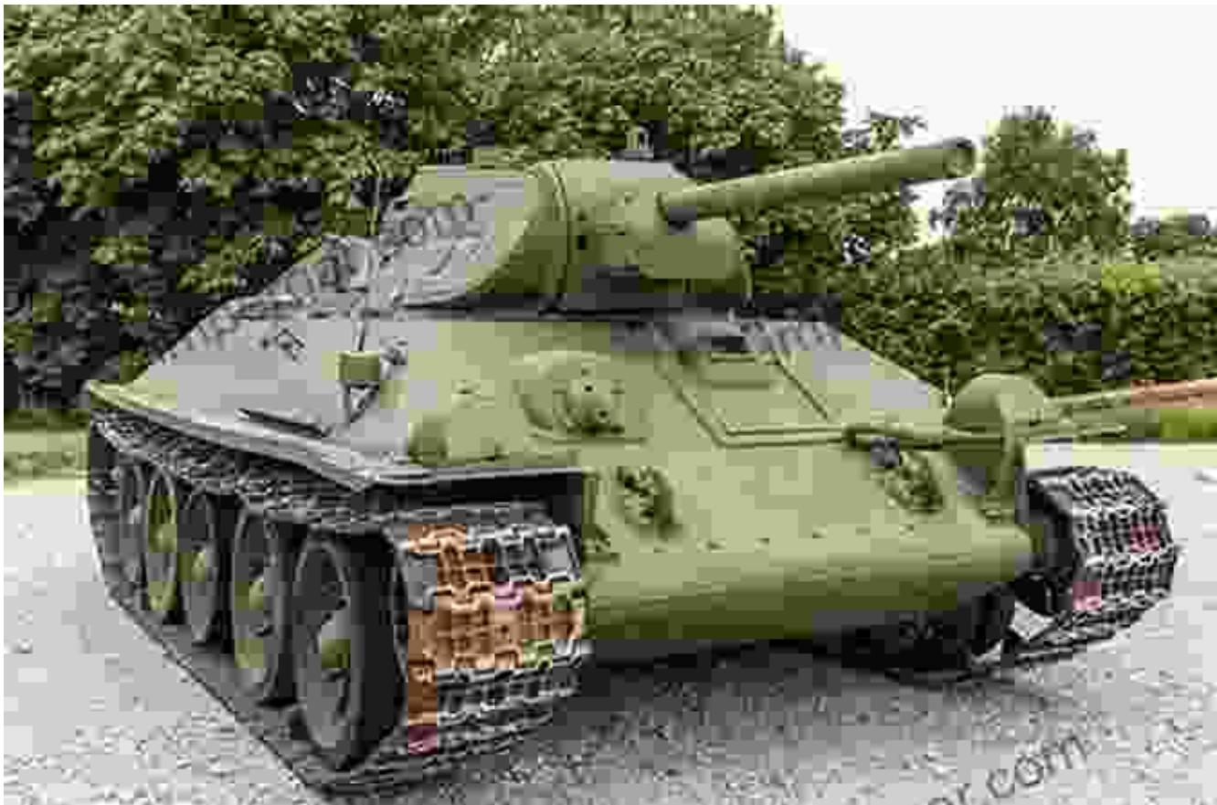
The T-34 was a Soviet medium tank renowned for its combination of firepower, mobility, and reliability. Its sloped armor deflected enemy shells, while its wide tracks and powerful engine provided excellent maneuverability.
